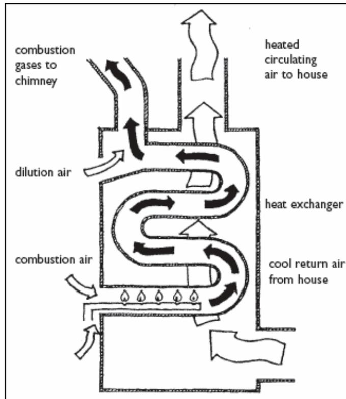
Figure 1: Basic Forced-Air Heating System Airflows
