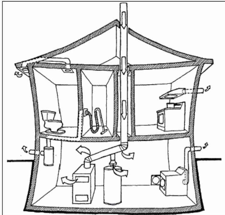
Figure 3: Backdrafting Due To Depressurization
